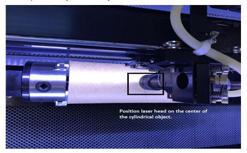
Tips: When installing the cylindrical object on the rotary, fasten it on the jaws. Be sure that both sides are secure in between the tapered cone and the jaws. Failure to keep the object balanced and secured on both ends on the rotary will result in uneven engraving.
